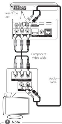
When you use COMPONENT VIDEO OUT connection, you can change the resolution for the output. (Refer to "Resolution setting" on page 17.)
